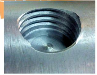
A mounting hole has been end-milled and bottomtapped into the sidewall of a pipe.
