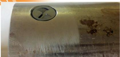
Close-up of an **STI** tag mounted into a pipe; notice that the tag is mounted flush to the surface of the pipe. Recessing the tag into the pipe deeper than shown may adversely affect the ability to interrogate the tag.
